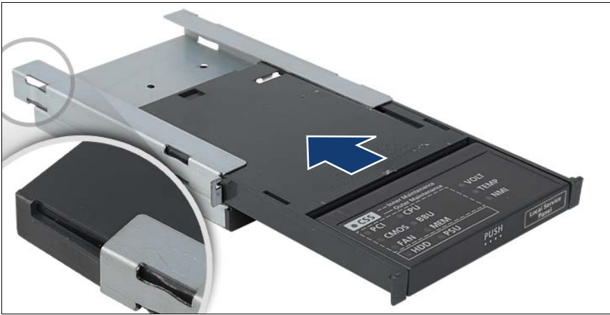
Figure 30: Sliding the LSP in the 3.5-inch frame
